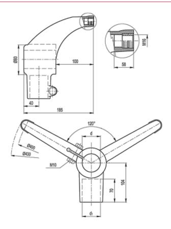
d (inch) = 1 1/2 Gas d1 (inch) = 1 1/4 Gas d1 (mm) = 42.4 d mm = 48.3 Weight (g) = 730
